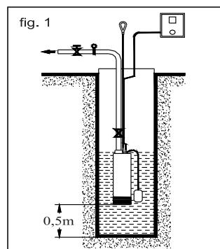
**WARNING:** It is advisable to install a gate valve at the pump output to avoid deposition and a check valve easily reachable to allow easy pump removal in cleaning and maintenance operations.
